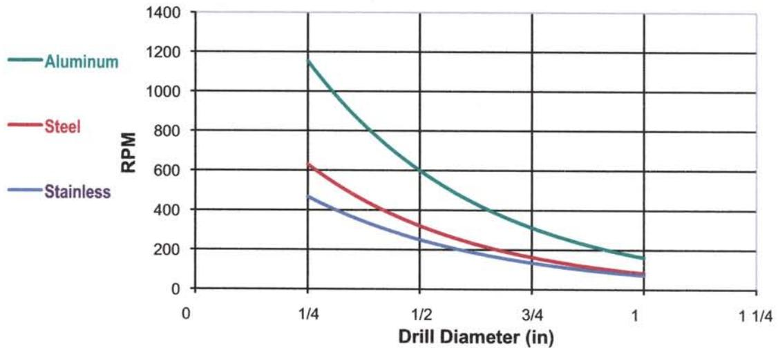
All holes 1/2" or greater should be drilled in 1/8" increments, starting with 3/8"
