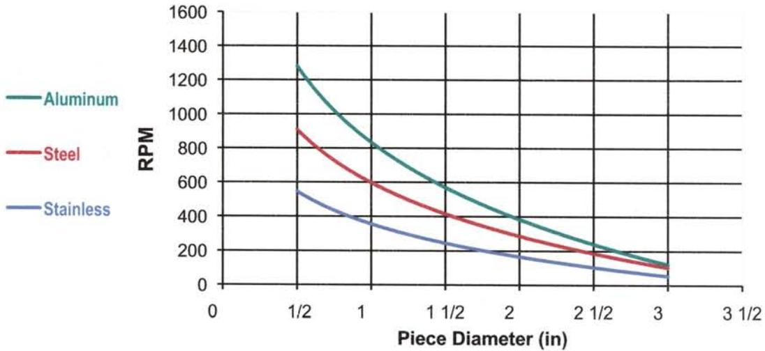
\*Knurling & parting tools are run at 100 RPM maximum
